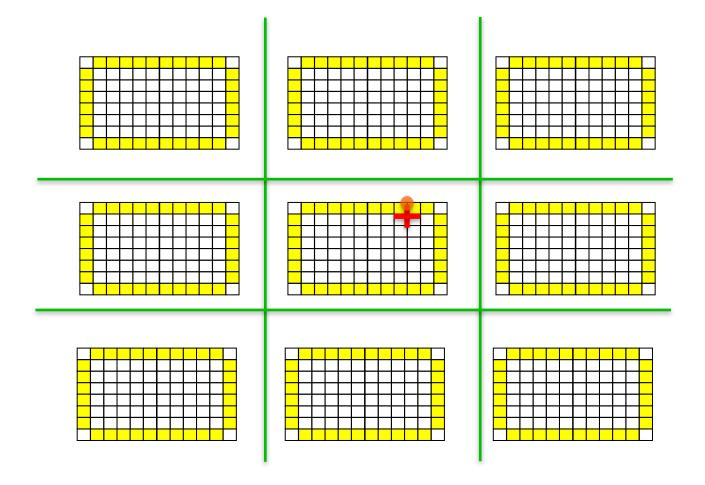
Provide access to remote data through a *halo* exchange (5 point stencil)
