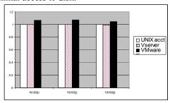
Figure 2: Comparison of different EFIT runs executing directly on Unix, under VServer and VMware. The times on Y axis are normalized to the Unix run.
