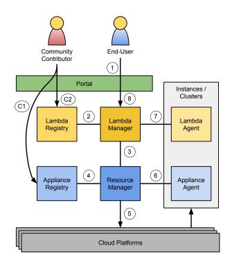
Figure 1: Diagram of the LambdaLink architecture
