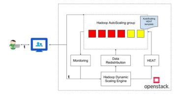
Fig. 1. Overview of the Hadoop dynamic scaling system
